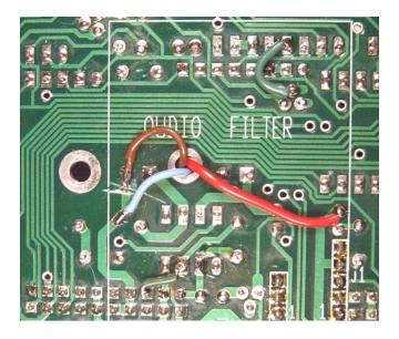
12 VDC can be taken from any point where it is convenient and the ground can be connected to any convenient point which is connected to the chassis ground. The figure above shows 12 VDC being taken from the 12 VDC side of R16 (see the schematic above) and the picture below shows the ground connection being tapped off Pin 4 or 5 of U9, both of which are grounded as shown in the schematic diagram:
